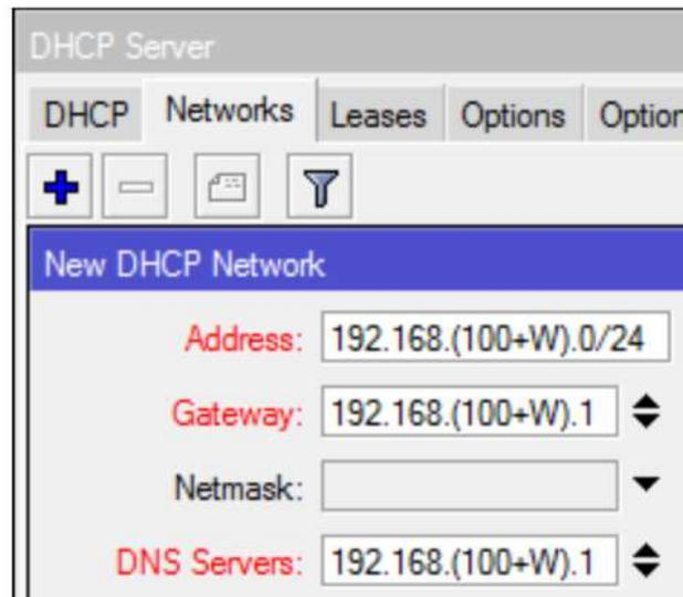
The screenshot shows the Mikrotik WinBox DHCP Server configuration window. The 'Networks' tab is active. A 'New DHCP Network' entry is being configured with the following fields:
